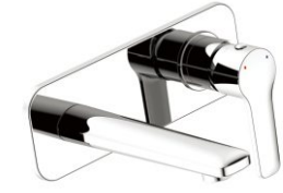
Item Nr. KC111700 Description Shower mixer • Brass body. Chrome plating. • Ø35mm ceramic cartridge.
